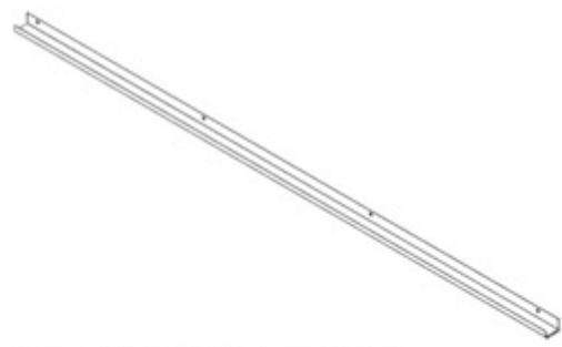
G04 GUTTER - A4M01999 (x2) 1 9/16"x1 15/16"x79 3/8" (40x50x2017)
